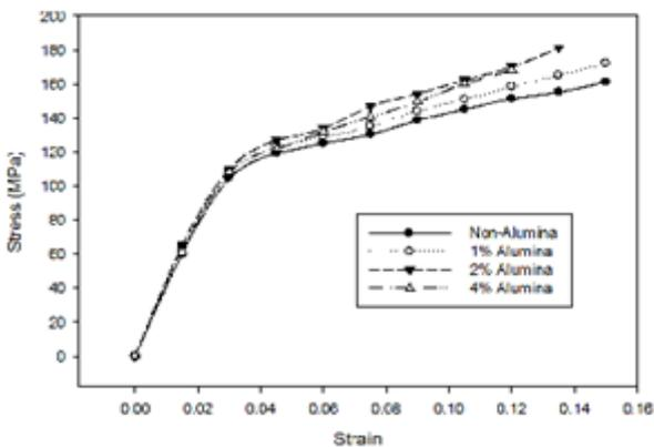
Fig. 3: Experimental flow stresses of AZ11 alloy with different weight percentages of 150(nm) nano- $Al_2O_3$  during the compression test.
