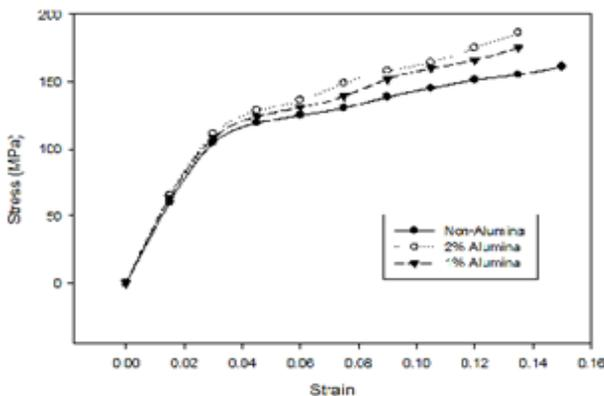
Fig. 4: Experimental flow stresses of AZ11 alloy with different weight percentages of 80(nm) nano- $Al_2O_3$  during the compression test.
