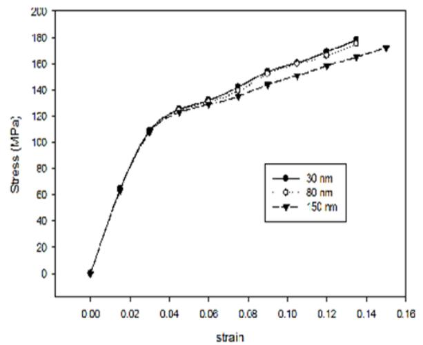
Fig. 6: Experimental flow stresses of AZ11 alloy with different sizes of vol. 1% nano- $Al_2O_3$  during the compression test.
