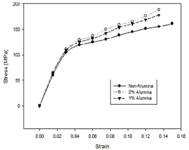
Fig. 5: Experimental flow stresses of AZ11 alloy with different weight percentages of 30(nm) nano- $Al_2O_3$  during the compression test.
