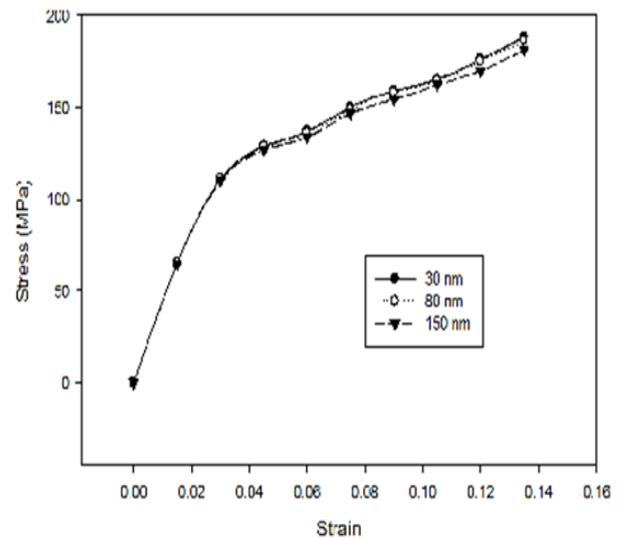
Fig. 7: Experimental flow stresses of AZ11 alloy with different sizes of vol. 2% nano- $Al_2O_3$  during the compression test.
